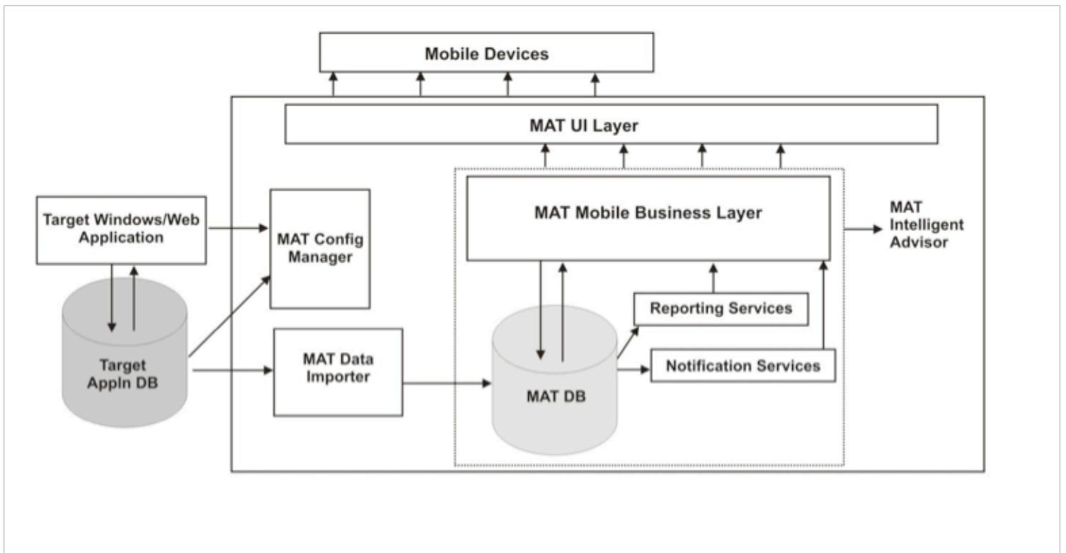
*Mobile Analytics Tracker (MAT), a mobile enabled website technology that allows users to access information in their palm literally. This plug and play software is hosted in the server and allows users to connect to the source database and access the information from anywhere. This is a must have technology for organizations that have their decision makers always on the go.*
